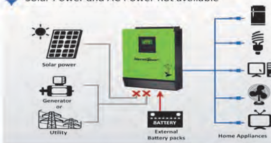
2 Solar Power and AC Power not available
